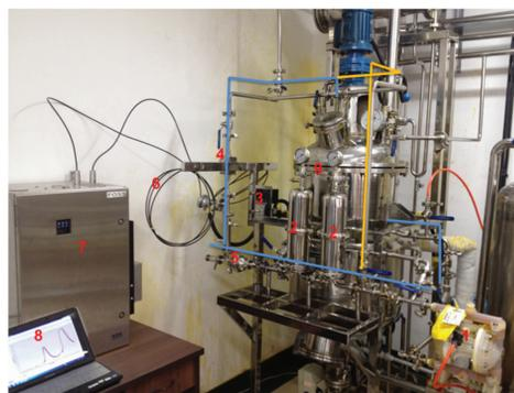
Fig. 1 Platform of on-line NIR
